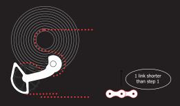
STEP 2: When tension is applied on the chain and the OSPW X System appears to be aligned as the diagram above, the chain needs to be cut (1 link shorter than step 1) and connected by the required amount of links in order to achieve sufficient tension in this gear combination (always the small cog on the cassette).
